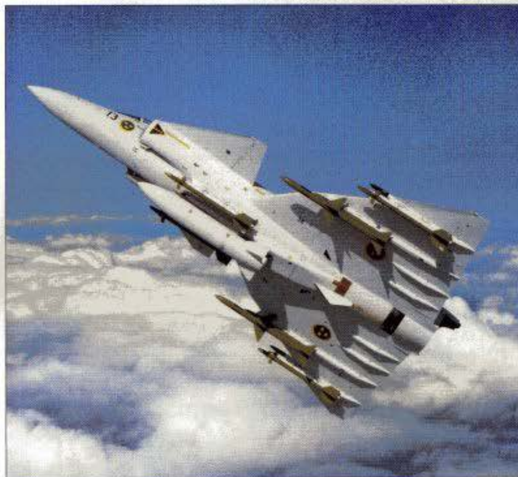
Above: The Viggen's large canard wing enables it to take off and land on very short runways. Below: A line-up of JA 37 Viggens from F17 at Kallinge in southern Sweden, some of them with the unique camouflage pattern chosen for most Swedish military aircraft. Lennart Berns.
